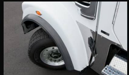
Wheel cut up to 50 degrees for excellent maneuverability.
